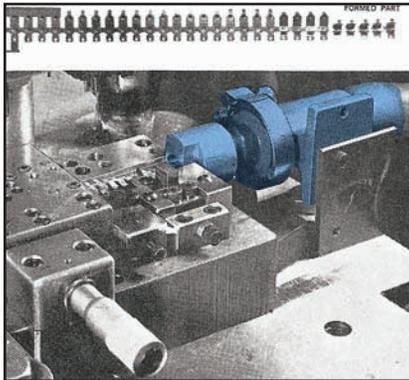
**PROBLEM:** Photograph shows the fabricating of a small formed part in a progressive die. The problem is to remove the finished part at the final cut-off station. The normal procedure is to use compressed air to blow this part into a container. Quite often this is inadequate as the parts could fly in various directions and often do not leave the die area. These parts would then interfere with the strip stock causing downtime or rejected parts.
