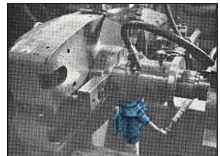
A VT-750-C1 Vacuum Transducer and Cap Unit was selected instead of a Vacuum Sleeve in order to accommodate any number of different dies. Otherwise, individual Vacuum Sleeves would have to be installed in each die. The "A" dimension of .750 insure sufficient clearance for all slugs.
