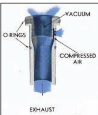
**SECTIONAL VIEW OF BAZOOKA VACUUM SLEEVE\*** illustrates how the metal scrap can pass through the sleeve without disrupting the vacuum flow or damaging the unit.
