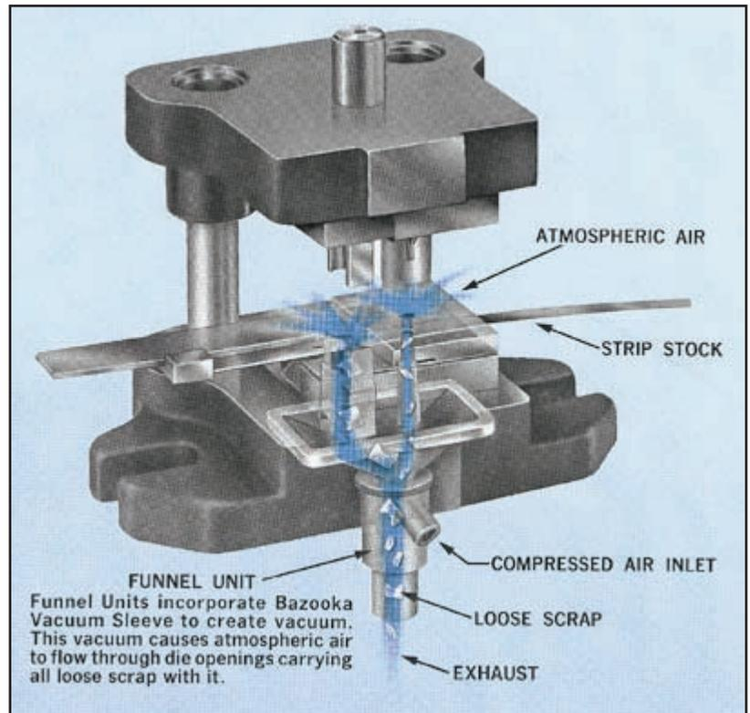
(C) **THE SOLUTION:** The BAZOOKA VACUUM SLEEVE was designed and developed as an easy method to remove loose slugs or scrap. The VACUUM SLEEVE will convert compressed air into a vacuum which is applied at the die opening. This vacuum not only **prevents slugs from pulling out with the punch, but it carries them away from the die surface** through the vacuum source and deposits them in a container.
